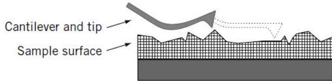
Sensor stage of an atomic-force microscope.
